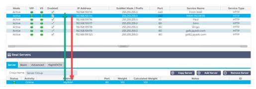
Once tested for threats, the data egresses from the WAF to the secondary VIP 192.168.159.115 and is then sent to the real server. The IP address 192.168.159.115 is entered in the Real Server/VIP field on the WAF, as illustrated in the image below.
