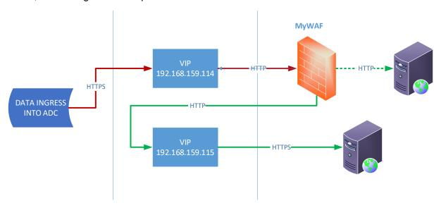
As we can see from the diagram above, data ingress occurs to the VIP 192.168.159.114 and is then sent onto the WAF. You will need to configure for SSL offload if the traffic is HTTPS – set the port for the ingress VIP to 443 and the port for WAF entry to 80 (our example).
