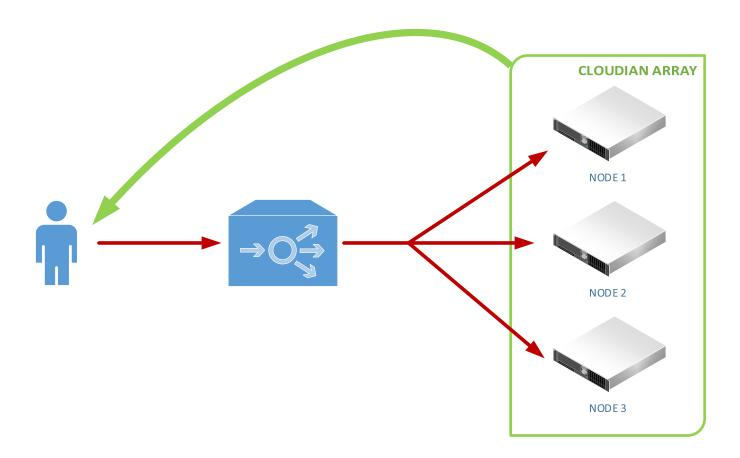
In the example shown, the Request traverses through the EdgeADC and is distributed to the Cloudian nodes using the load balancing policy.
