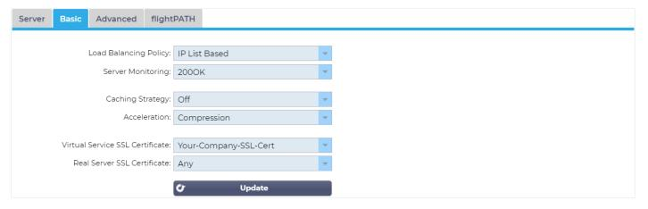
The above configuration will ensure SSL offload and re-encryption. Should you not require this, we would suggest as follows:
