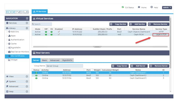
You will note that we have kept the Dashboard VIP on Layer 7 HTTP. The reason for this is that you may wish to use flightPATH based filtering to limit access to the VIP by country, or Source IP, or even a series of subnets based using RegEx.
