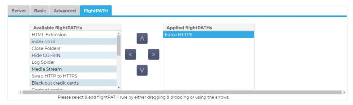
The flightPATH rule is now activated, and all traffic entering the VIP on port 80 will be switched to use the 443 based VIP.
