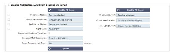
There are several types of event notifications that the ADC will send to persons configured to receive them. You can tick and enable the notifications and alerts that should be sent out. Notifications occur when Real Servers are contacted or channels started. Alerts occur when Real Servers cannot be contacted, or channels stop working.
