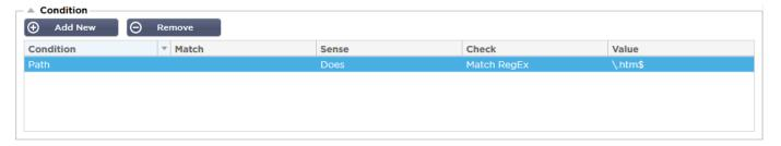
You can also use RegEx by selecting Match RegEx in the Check field and the RegEx value in the Value field. The inclusion of RegEx evaluation extends the capability of flightPATH tremendously.
