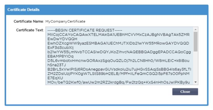
You will need to cut and paste the contents into a TEXT file and name it with a CSR file extension, for example, *mycert.csr*. This CSR file will then need to be provided to your certificate authority to create the SSL certificate.
