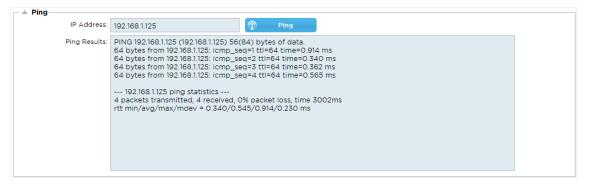
Type in the host's IP address you wish to test, for example, the default gateway using dotted decimal notation or an IPv6 address. You may have to wait a few seconds for the result to feedback once you have pressed the "Ping" button.
