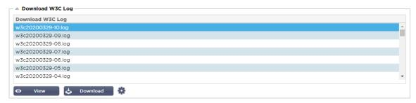
W3C logging is enabled from the System > Logging section. A W3C log is an access log for Web servers in which text files are generated containing data about each access request, including the source Internet Protocol (IP) address, the HTTP version, the browser type, the referrer page, and the timestamp. W3C logs can become very large depending on the amount of data and the category of logging being recorded.
