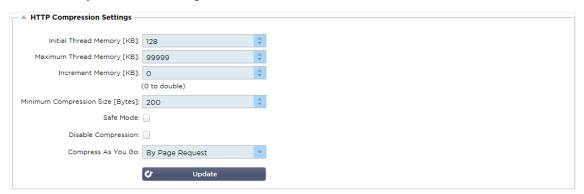
Compression is an acceleration feature and is enabled for each Service on the IP Services page.
