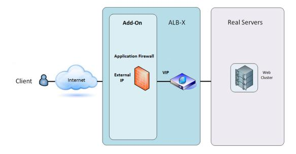
In this architecture, only HTTP can be used for your service as the Firewall cannot inspect HTTPS traffic.
