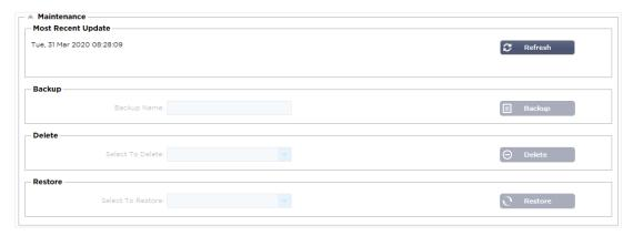
This section will be greyed out if you have enabled historical logging. Please untick the Enabled checkbox in the Collect Data section and click Update to allow the maintenance of the historical logs.
