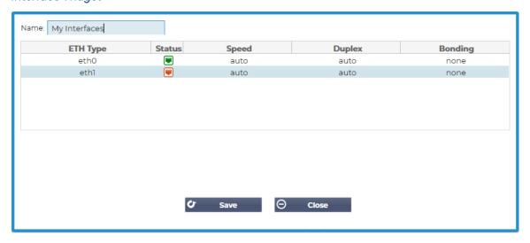
The Interface widget allows you to display the data for the chosen network interface, such as ETH0, ETH1, and so on. The number of available interfaces for addition depends on how many network interfaces you have defined for the virtual appliance or provisioned within the hardware appliance.
