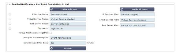
There are several types of event notifications that the ADC will send to persons configured to receive them. You can tick and enable the notifications and alerts that should be sent out. Notifications occur when Real Servers are contacted or channels started. Alerts occur when Real Servers cannot be contacted, or channels stop working.
