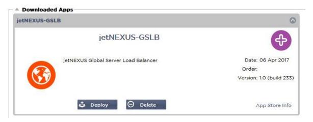
Following installation, please configure GSLB Add-On details, including Container name, External IP and External Ports in the Library > Add-Ons page of the ADC GUI as shown in the figure below.
